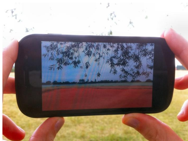
Figure 5: BGS iGeology 3D 'augmented reality' Smartphone app for displaying the geological map over the landscape
