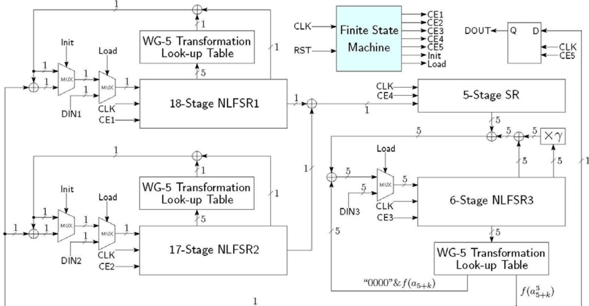
Figure 3. The Data Path of the Lightweight PRNG Core
