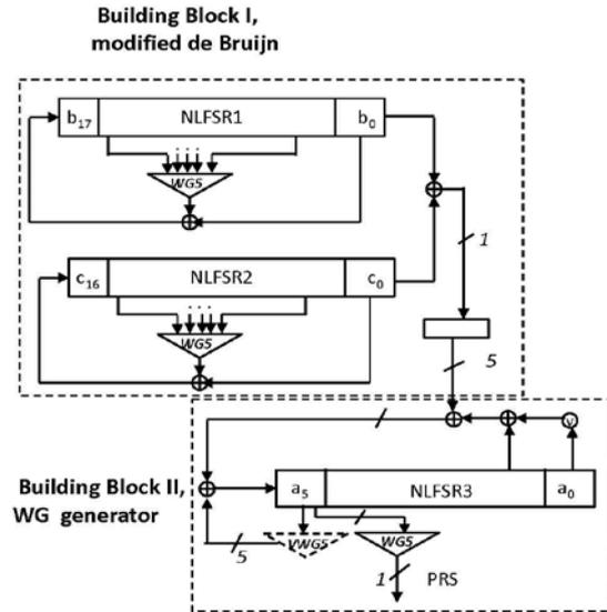
Figure 2. A Diagram of the PRNG for EPC C1 Gen2 Tags
