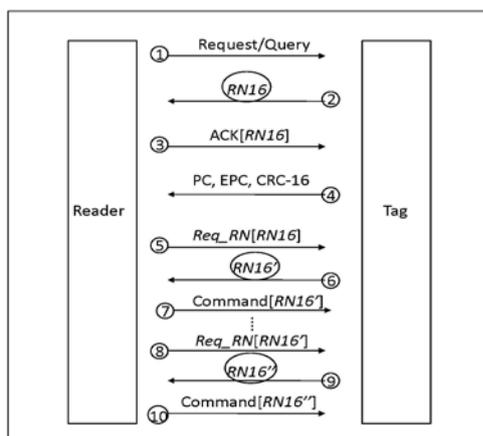
Figure 1. EPC C1 Gen 2 Tag Identification Protocol
