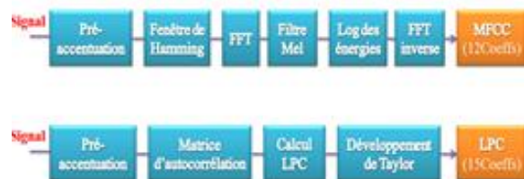
Figure 1. Illustration of flowchart to compute LPC and MFCC features
