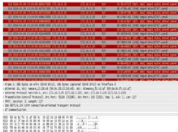
Figure 11. Traffic between HMI and adversary machine during launched DoS attack
