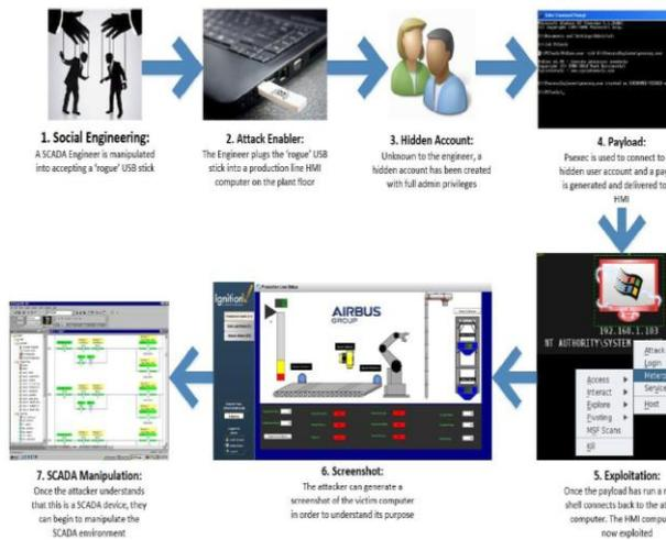
Figure 5. The attack flow scenario utilising a USB device
