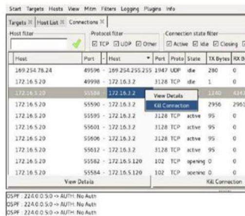
Figure 4. Killing target connections using Ettercap
