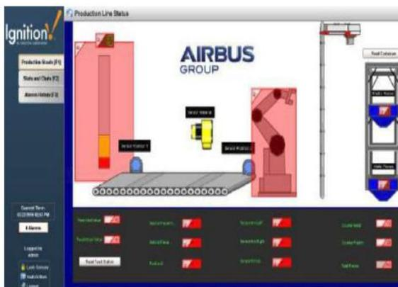
Figure 10. Visual indicator that the production line HMI has been disrupted
