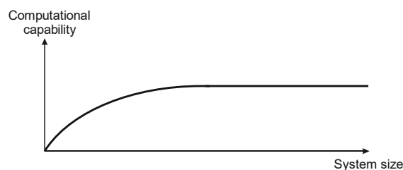
Figure 2. The size-related saturation of computational capability for a physically large system
