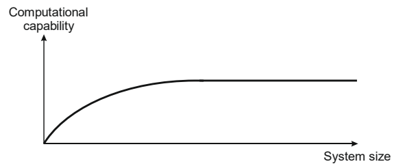
Figure 2. The size-related saturation of computational capability for a physically large system
